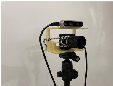
Fig. 4. Multiple camera system for data acquisition, with the RealSense D435i on top and CeleX-V below.
