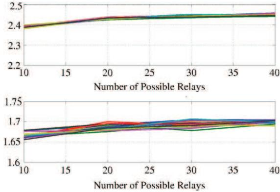
**Fig. 9.** Duration of the selection process (expressed in number of time-slots) as a function of the number of relay terminals  $N$ : average number (top) and standard deviation (bottom) for different values of the scale parameter.
