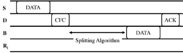
Fig. 5. Frame exchange sequence in the protocol using the basic IEEE 802.11 access method ( $S$  is the source terminal,  $D$  is the destination terminal,  $B$  is the best relay terminal, and  $R_i$  is a relay candidate).
