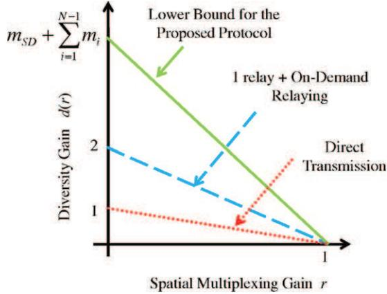
Fig. 6. DMT curves of three protocols: the proposed protocol, the direct transmission, and the on-demand cooperation with one relay terminal [6]. For the special case of Rayleigh fading,  $m_{SD} + \sum_{i=1}^{N-1} m_i = N$ .
