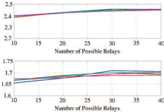
**Fig. 10.** Duration of the selection process (expressed in number of time-slots) as a function of the number of relay terminals  $N$ : average number (top) and standard deviation (bottom) for different values of the shape parameter.
