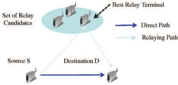
Fig. 1. Cooperation scenario with three relay terminals.
