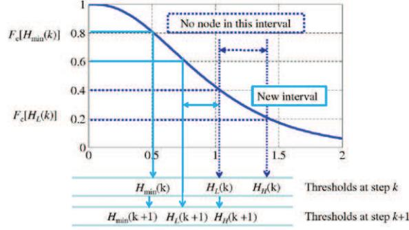
Fig. 4. Threshold adjustments of the splitting algorithm at terminal  $R_i$  when the feedback is 0 (idle) and a collision has occurred in the past.
