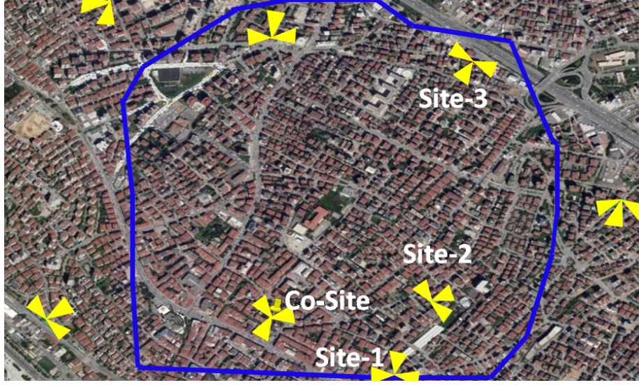
Figure 2: Locations of experimental sites in Turkey with 2 external FDD based MIMO sites (site-1 (800 Mhz band), site-2 (1800 Mhz band) and site-3 (2600 Mhz band)) all operating in 10 Mhz bandwidth and co-sites with TDD-based massive MIMO and FDD based MIMO (800 Mhz band and 10 Mhz bandwidth, 1800 Mhz band and 20 Mhz bandwidth).
