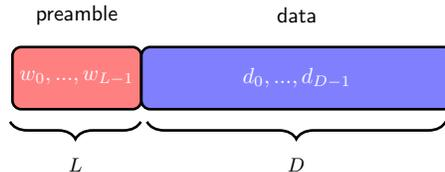
Figure 2: Packet structure of length  $P$ :  $L$  preamble symbols and  $D$  data symbols,  $P = L + D$ .
