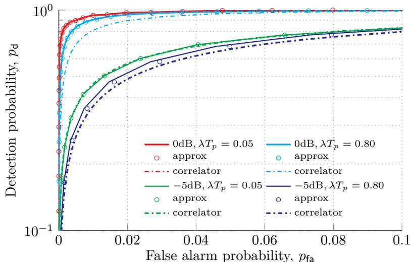
Figure 4: ROC for LRT-based detection for different SNR and traffic intensities. Results of the exact expression leaning on the probabilities given in Table 2 are reported by solid lines and circle markers lean on the approximation in (12). Dashed lines indicates the correlator performance. In all cases, the preamble length is of  $L = 16$  symbols while data is  $D = 256$  symbols long.
