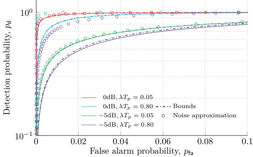
Figure 3: ROC for correlation-based detection for different SNR and traffic intensities. Results of the exact expressions in (5) and (6) are reported by solid lines while dashed lines corresponds to the bound of  $p_{fa}$  in (10). Circle markers indicate performance estimated neglecting the presence of data and considering only false alarms due to noise. In all cases, the preamble length is of  $L = 16$  symbols while data is  $D = 256$  symbols long.
