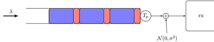
Figure 1: Queue system model: the arrival Poisson rate  $\lambda$  and service time  $T_p$ .
