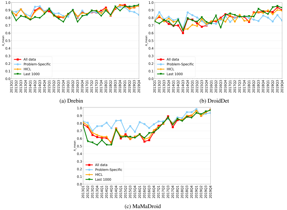
Figure 6: Evolution of the performance of malware detectors with periodic retraining for the period 2013-2019. Red lines represent the performance when using all the data available, i.e., the baseline. Green, blue and orange lines represent respectively the performance of models when retrained with the 1000 most recent samples, using the problem-specific strategy and with the HICL selection methods with labeling budgets of 70%.
