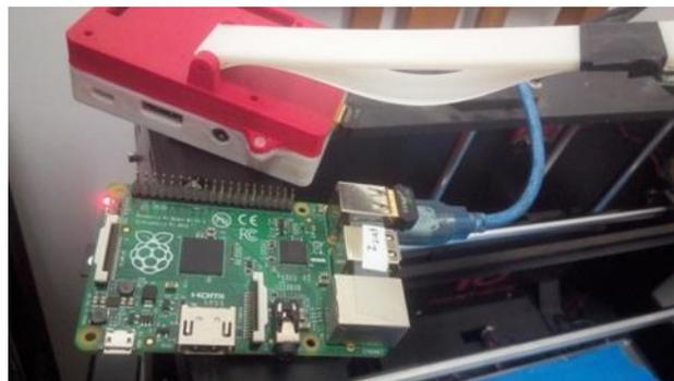
(a) A cloud access adapter for FDM 3D printers.
