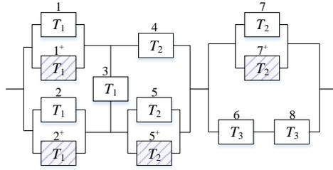
Figure 3: Reliability block diagram of the optimized system in example 1
