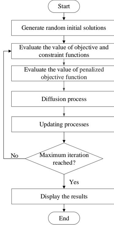
Figure 1: Procedure for optimization for RRAP
