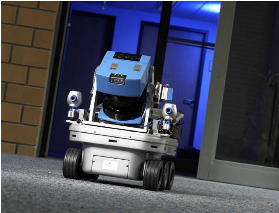
Fig. 1. The mobile robot Kurt3D, equipped with AIS 3D laser scanner.
