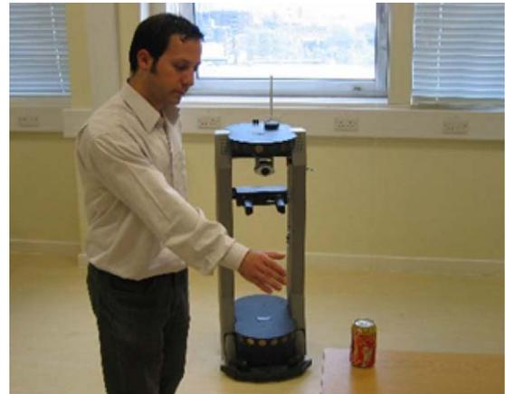
Fig. 3. The experimental setup involves an ActivMedia Peoplebot observing a human demonstrator acting on objects.
