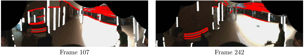
Figure 19: Panoramic representation of several full-rectified frames. Vertical lines are shown in white and horizontal ones in red. The horizontal vanishing point is aligned to the image center.
