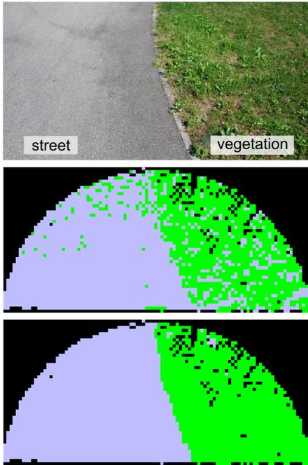
Figure 1: A street and an area containing grass (top) and typical classification results obtained based on range differences (middle) and remission values (bottom). Shown is a bird’s eye view of a 3D scan of the area depicted at the top with a maximum range of 5 m. Whereas points classified as street are depicted in blue, points corresponding to vegetation are colored in green.
