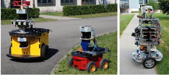
Figure 10: Robots used in our experiments. Left: An ActiveMedia Powerbot (yellow) and a Pioneer2 AT (red). Right: the EUROPA platform.
