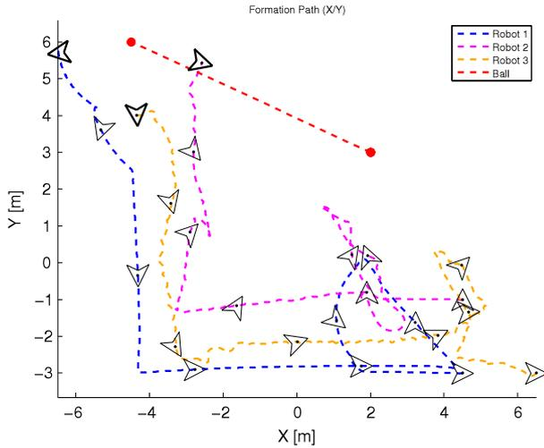
Fig. 3. The problem simulation: Formation behavior without the TSTFA approach.
