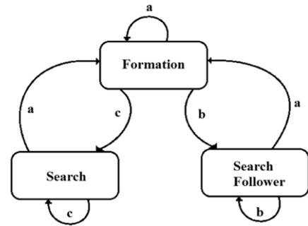
Fig. 1. Robot state machine.
