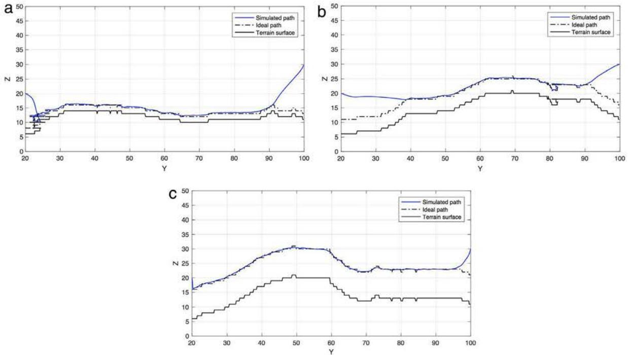
**Fig. 8.** Comparison of the resulting path against the ideal path and the profile terrain: (a) path at flight level 2; (b) path at flight level 5; (c) path at flight level 10.
