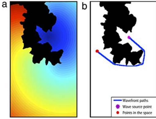
Fig. 2. Application of the FMM: (a) the time of arrival map; (b) the resulting path in the initial map.
