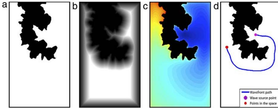
Fig. 4. Application of the FM<sup>2</sup> method: (a) map read as binary gridmap; (b) the Velocities map  $F$ ; (c) the time of arrival map  $T$ ; (d) the resulting path in the initial map.
