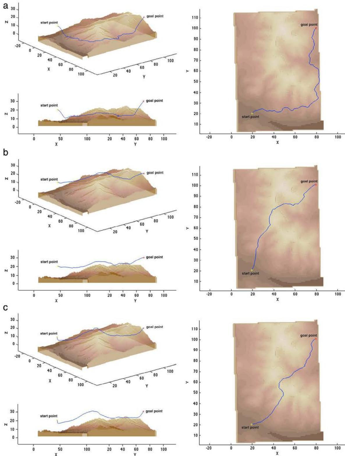
Fig. 7. Paths at different flight levels with respect to the ground: (a) path at flight level 2; (b) path at flight level 5; (c) path at flight level 10.
