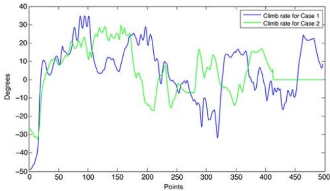
Fig. 12. Profile of the climb angle for different smoothness of the trajectory.
