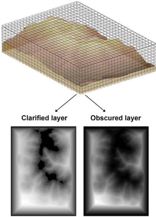
Fig. 6. The upper part of the image shows the 3D grid map of the environment. The lower part shows clarified and obscured layers of the map  $F$ .
