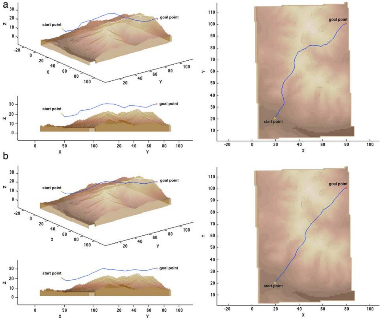
Fig. 9. Paths at flight level 10 with different smoothness: (a)  $p_1 = 0.5$  and  $p_2 = 1$ ; (b)  $p_1 = 0.5$  and  $p_2 = 0.8$ .
