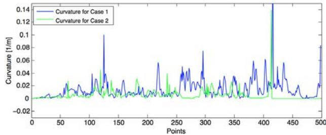
Fig. 13. Profile of the curvature for different smoothness of the trajectory.
