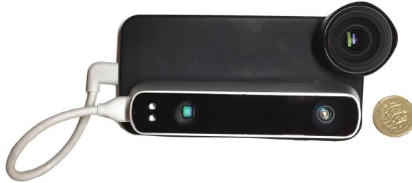
Figure 11: Mobile RGB-D capture setup used in this work. An Occipital Structure sensor is used to collect depth while RGB is collected by a wide-angle lens (Moment wide lens) mounted on an iPhone camera. The effective angle-of-views are respectively  $85^\circ \times 70^\circ$  and  $58^\circ \times 45^\circ$  for the color and the infrared camera and the baseline between them is around 38 mm. Both cameras operate at 30 fps with VGA resolution.
