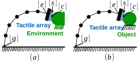
Figure 5: Physical interactions. A robot with a pressure sensing array interact with: (a) the stiff environment and (b) an object on the stiff environment. The frames  $\{g, e, s, c\}$  correspond to the global, end-effector, sensor, and contact coordinate frames.
