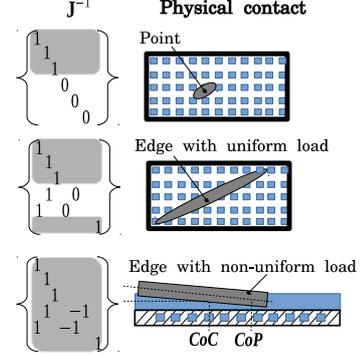
Figure 7: Illustration of elements of the touch-dependent tactile Jacobian for three physical contacts: point, edge, and edge with non-uniform load. The shaded rows in  $\mathbf{J}^{-1}$  of every contact type contribute to the robot end-effector pose.
