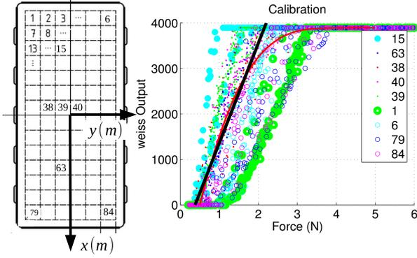
Figure A.15: Responses of the individual sensor elements to the applied forces on each element. The sensor outputs are the raw values that are proportional to the (resistance) voltage: the WEISS WTS 0614 sensors use piezoresistive technology.
