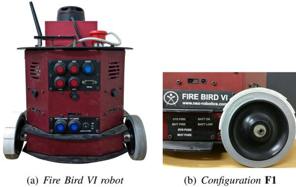
Fig. 2. One of the wheels (left) of *Fire Bird VI* robot is deformed such that the wheel loses its notion of circularity.
