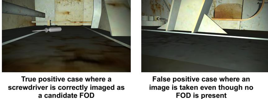
Figure 8: Examples of candidate FOD photos, taken by the inspection robot, that are shown to remote humans for final decision-making.
