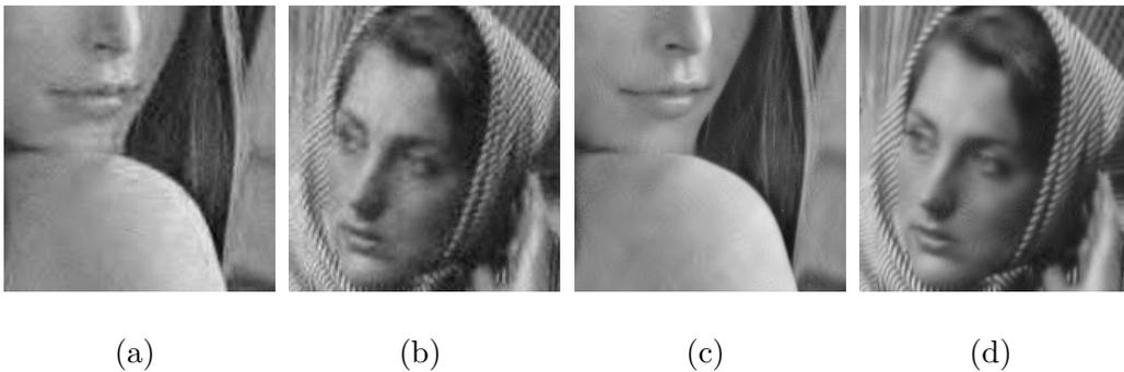
Fig. 16. Denoising results of the fragments of Lena and Barbara test images corrupted by zero-mean AWGN with  $\sigma_Z^2 = 400$  when side information information about edge coefficient positions and means is available: (a) and (b) DWT domain set-up; (c) and (d) DOT domain set-up.
