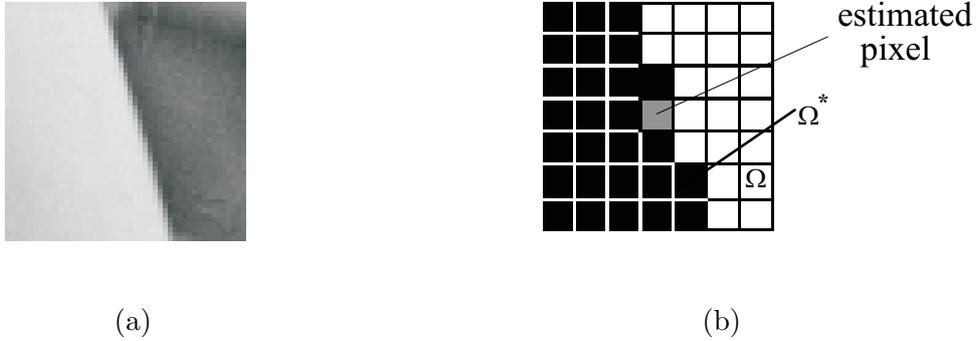
Fig. 4. (a) Fragment of test image Lena; (b) local estimation window with indication of the subset (black pixels) and of the estimated pixel (gray) for the restricted support ML local variance estimation.
