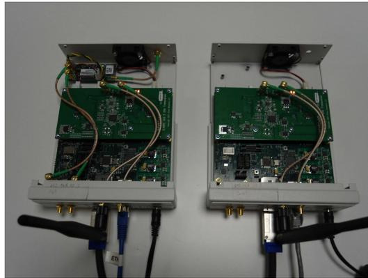
Figure 10: N210 Ettus devices with the XCVR2450 daughterboard installed. A two-antenna cognitive receiver is composed of two N210 boards connected through a MIMO cable.
