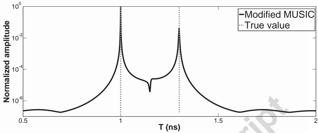
Figure 6: Case 1, Pseudo-spectrum of MUSIC for time delay estimation with SNR=20 dB, the two time delays are 1 ns and 1.3 ns in grey dashed line, slightly overlapped.
