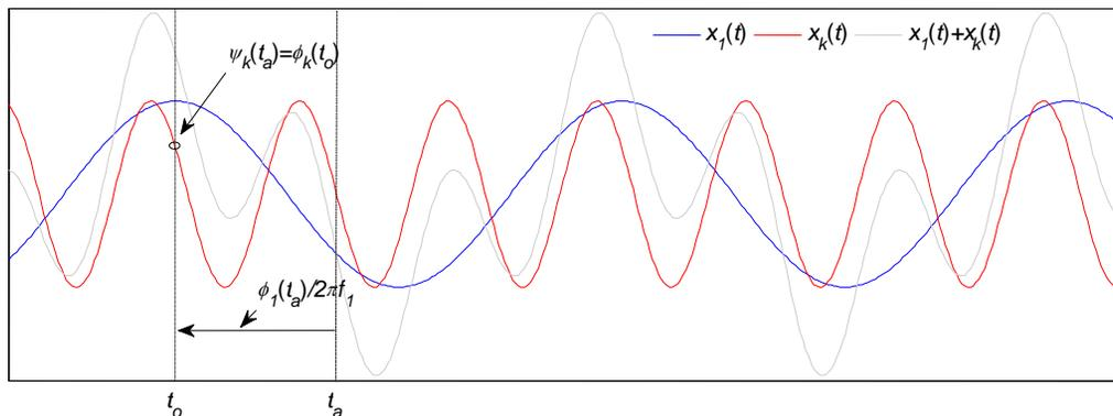
Figure 1: Graphical interpretation of the RPS transformation: for an analysis instant  $t_a$  the RPS of  $k$  is the phase shift of that component with respect to the fundamental component at the point where the period of the fundamental component starts ( $t_0$ ).
