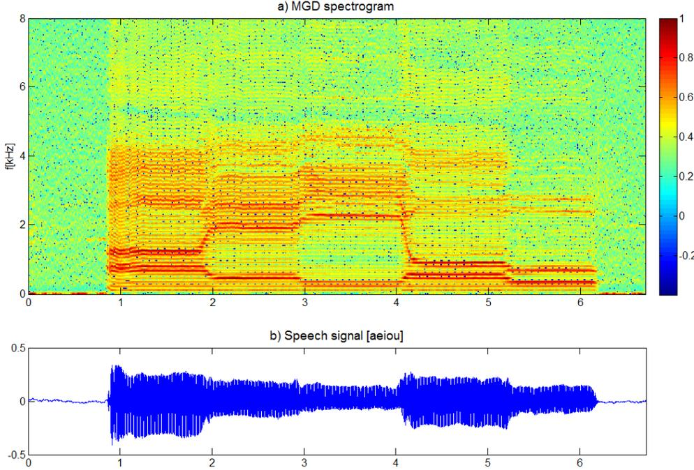
Figure 3: MGD spectrogram of a voiced speech segment with five continuous vowels.
