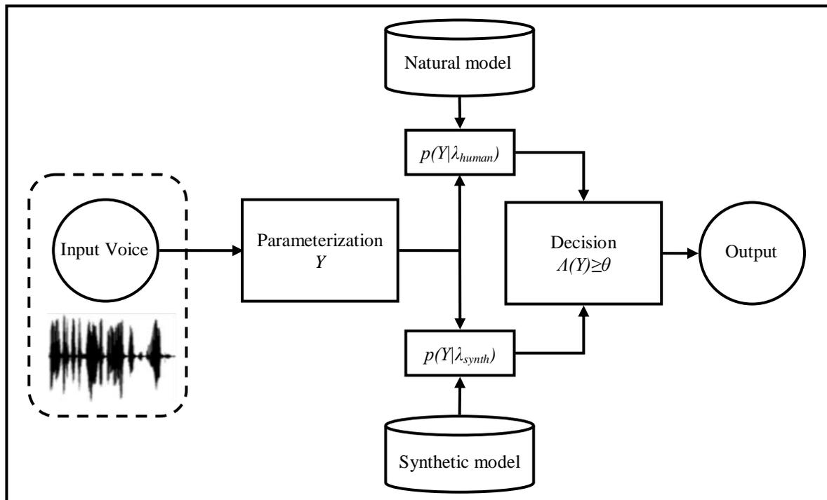
Figure 4: SSD system structure.
