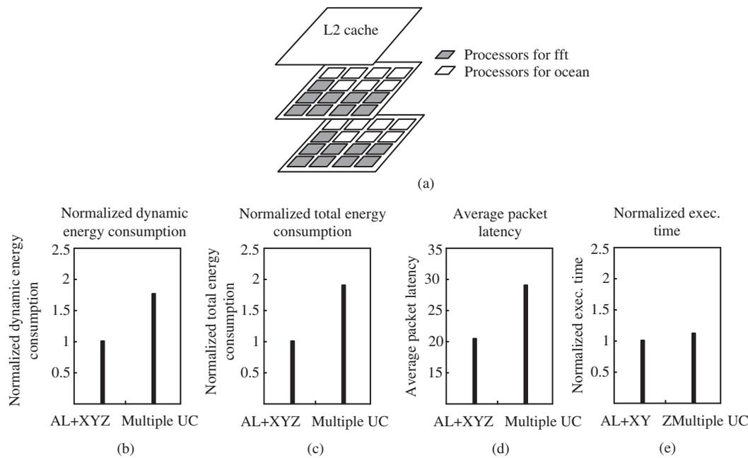
**Fig. 21.** (a) Two sub-networks in a different NoC architecture. An L2 cache is placed in a separate layer. The other tiles are composed of processors, L1 caches, and routers. Normalized dynamic energy consumption (b), total energy consumption (including both dynamic and leakage power) (c), latency (d), and normalized execution time (e) of AL + XYZ and Multiple UC.
