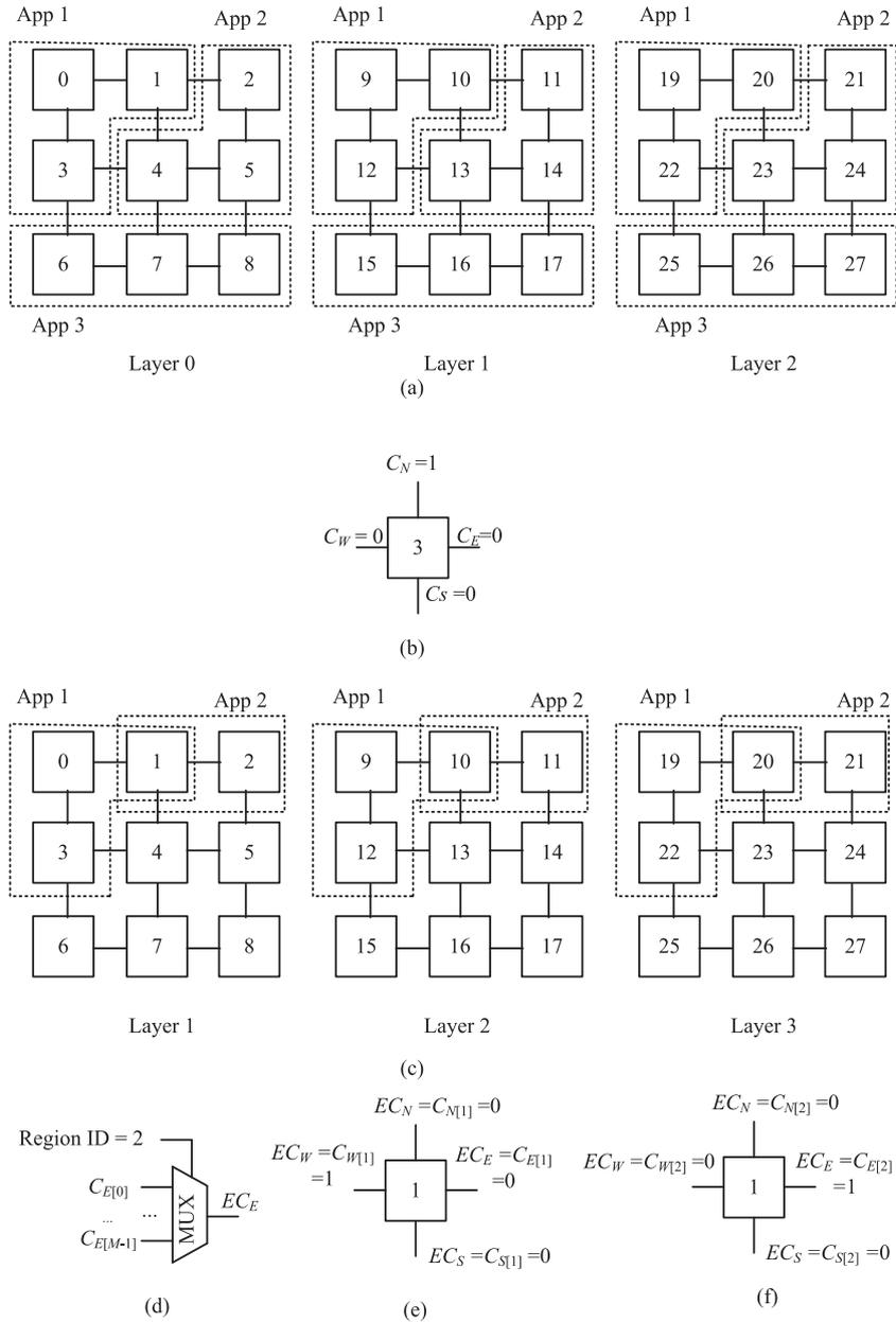
**Fig. 10.** (a) Sub-networks with 3 applications mapped on. (b) Connectivity bits of node 3. (c) Two overlapped sub-networks sharing node 2. (d) Extended connectivity bit generated using a MUX. (e) Extended connectivity bits of node 1 for Sub-network 1 in (c). (f) Extended connectivity bits of node 1 for Sub-network 2 in (c).
