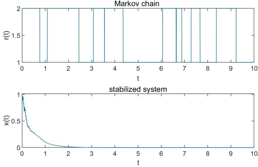
Figure 4.1: Simulated path of Markov chain  $r(t)$  and state  $x(t)$ , by the Euler–Maruyama method with step size  $10^{-6}$ , observation interval  $\tau = 0.00045$  and random initial values.
