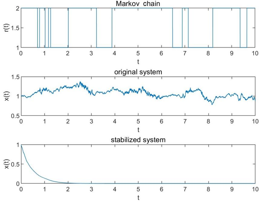
Figure 4.2: Simulated paths of the system mode and state. The upper plot shows the Markov chain  $r(t)$ , the middle and lower plots respectively show the state  $x(t)$  of the original system and the stabilized system. The Euler–Maruyama method with step size  $10^{-6}$  and random initial values have been used.
