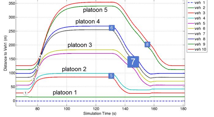
Figure 13: Effect of changing  $optPlnSize$  at  $t=73s$  from 10 to 2 on a 10-vehicle platoon. The platoon management protocol attempts to meet the new platoon size by performing four splits one after the other (as marked from 1 to 4). At  $t=130s$ , the  $optPlnSize$  is changed back to 10, and four merges (marked from 5 to 8) are performed to form a 10-vehicle platoon.
