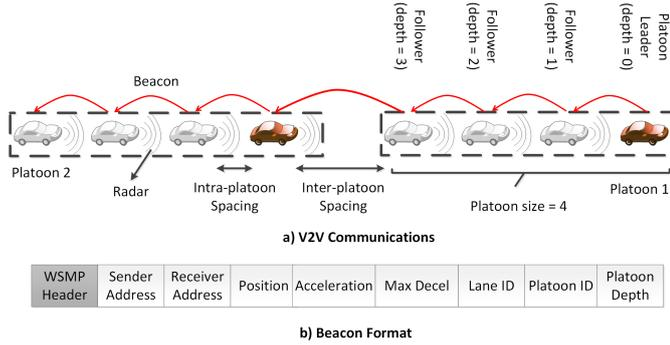
Figure 2: One-vehicle look-ahead communication in CACC platoon.  $i$ th vehicle receives information embedded in beacon messages from  $(i - 1)$ th vehicle using V2V wireless communication and feeds it into the longitudinal control system (detailed in Section 3.3) to maintaining a safe gap from the preceding vehicle. All vehicles are equipped with radar to measure the space-gap and velocity of the preceding vehicle.
