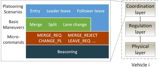
Figure 1: Platoon management protocol resides in the coordination layer of each vehicle and uses wireless V2V communication to exchange micro-commands between neighboring vehicles in order to coordinate different maneuvers.
