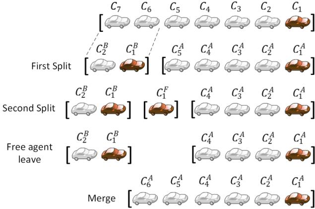
Figure 8: Following vehicle  $C_5$  decides to leave the platoon (leaders are shown in red). Platoon leader  $C_1$  issues the first split maneuver to split the platoon after  $C_5$ . Then it issues the second split maneuver to make  $C_5^A$  a free agent.  $C_1^F$  exits, and the two platoons are merged afterward, and the gap is closed.
