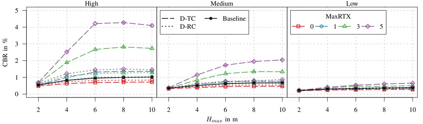
Figure 11: Mean CBR for different  $H_{\max}$  and MaxRTX values, and for different vehicular density scenarios (LuST).
