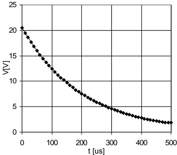
Fig. 11: Resulting course of simulation for 11 diodes in chain.
