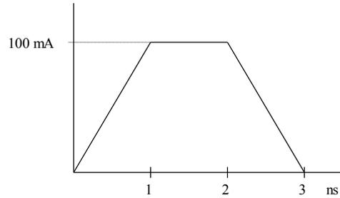
Fig. 4: Simulated shape of the current pulse at breakdown
