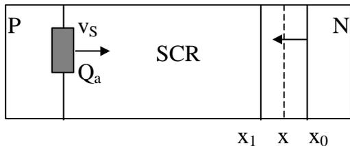
Fig. 2: Scheme of local avalanche breakdown
