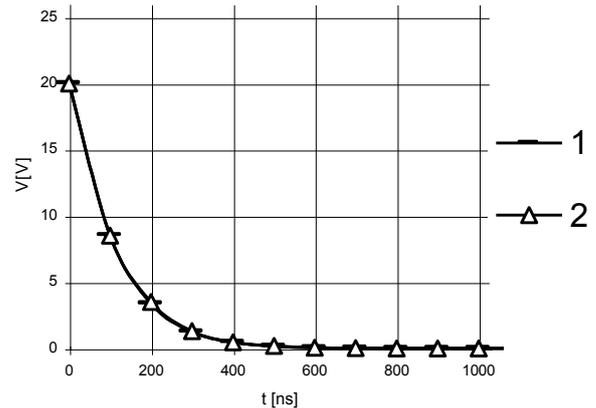
Fig. 5: Calculated dependencies of the voltage change after finish of breakdown (physical analysis 1 vs. circuit computer simulation 2)
