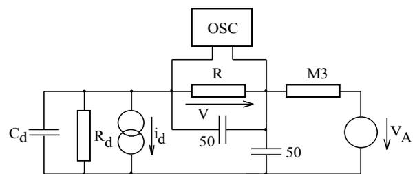
Fig. 8: Substitute scheme of measuring circuit
