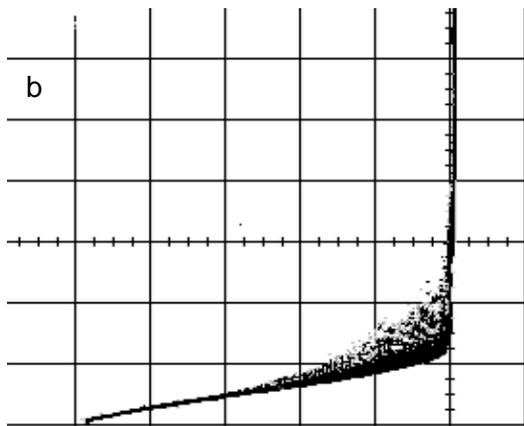
Fig. 6a, b: Examples of experimental I - V reverse characteristics (with breakdown noise); repeated frequency is 0,02 Hz, time measurement about 100 s
