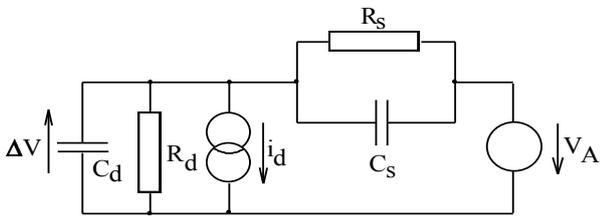
Fig. 10: Substitute circuit for HVDS
