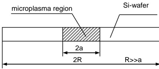
Fig. 12: Silicon wafer with microplasma "hot spot"
