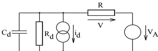
Fig. 3: Individual diode in simulated circuit
