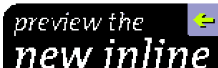
Figure 3-3: Converted to JPEG, quality factor = 1
