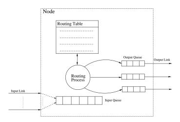
Fig. 5. Simulation Model for DVR
