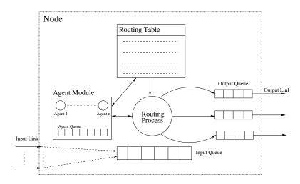
Fig. 6. Simulation Model for ADVR
