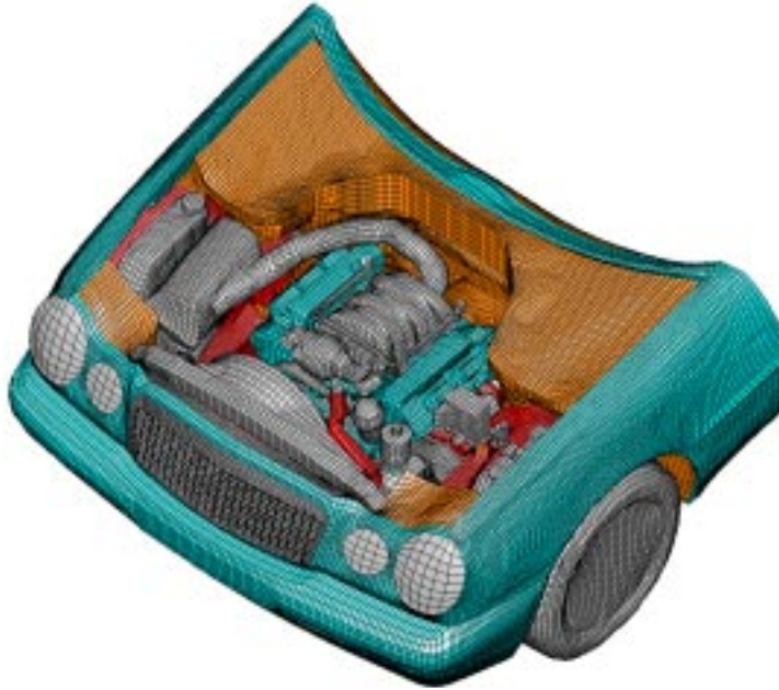
Figure 1: Mesh for computing the underhood flow of a Mercedes-Benz E-Class
