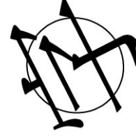
Fig. 8. The crossing counts of the strokes and the circle is rotation invariant.
