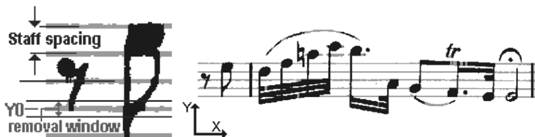
Fig. 2. Staff lines removal (removed pixels in light gray).
