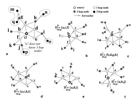
Fig. 2. Network example: (a) Node *a* knows its two-hop neighborhood, and the *one-hop dominating nodes* (i.e.,  $D_{1-hop}$ ) selected by each one-hop neighbor. A subset of nodes from  $\bigcup_{n_j \in N_i} D_{1-hop}^j$  (i.e.,  $\{g, h, i, j\}$ ) cover all nodes in the three-hop neighborhood of node *a*. (b–f) show the network from the point of view of each neighbor of node *a*, and how each  $D_{1-hop}$  list is obtained via DP.
