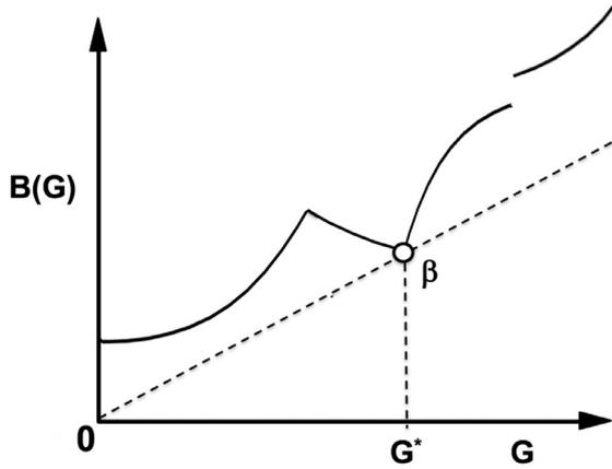
(b) Non-differentiable, Non-convex, Discontinuous  $B(G)$ .Fig. 9. Finding the optimum operating Point  $G^*$ .
