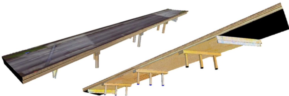
Figure 1: 3D as-is model of fully-textured RC highway bridge, deck view on the left, bottom view on the right
