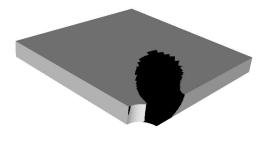
Figure 10: Elastic (gray color) and plastic (black color) elements at time  $t_8\,$
