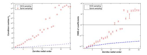
Figure 2: Left: condition number  $\kappa_2$  of the collocation matrix (5) as a function of the radial order, for both the spiral pattern and the OCS. Right: range plot of the RMS error of the recovered Zernike modes with respect to the exact coefficients.
