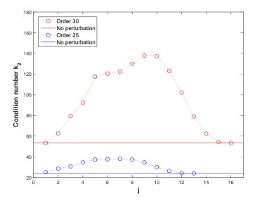
Figure 4: Maximal change in the condition number when a single circle of radius  $r_j$  is rotated,  $1 \le j \le k(n)$ , for radial orders n = 25 and n = 30.
