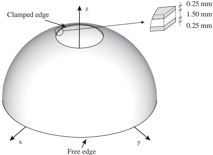
Figure 11. Hemispherical sandwich shell with a hole.
