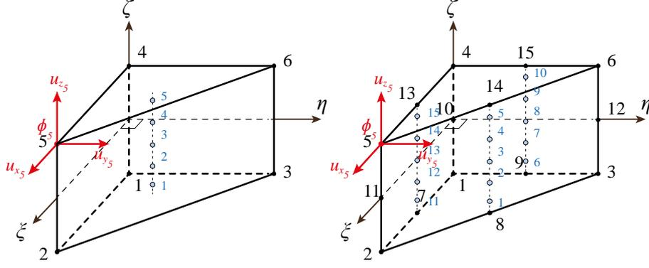
Figure 1. Schematic representation for the reference geometry of the SHB6E and SHB15E elements as well as for the location of their integration points in the case when the number of through-thickness integration points is  $n_{\text{int}} = 5$ .
