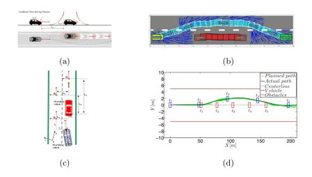
Figure 5: Trajectory planning via (a) Potential Fields [43]; (b) RRT [63]; (c) Virtual Reference Tracking [5]; (d) Model Predictive Control [47]
