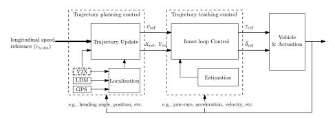
Figure 4: General control architecture for an autonomous vehicle [38, 43, 49–51]. (V2X block with dot-dash boundary: optional functionality)
