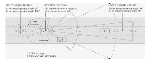
Figure 2: Visibility of an autonomous vehicle. **Note:** SV: Subject Vehicle, TV: Traffic Vehicle. Sensor performance specifications are based on [34]
