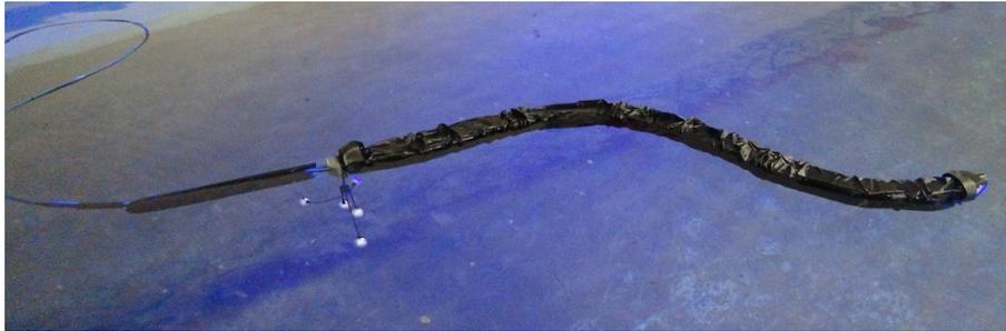
(b) Underwater snake robot Mamba with a passive caudal fin attached to the last module of the robot.
