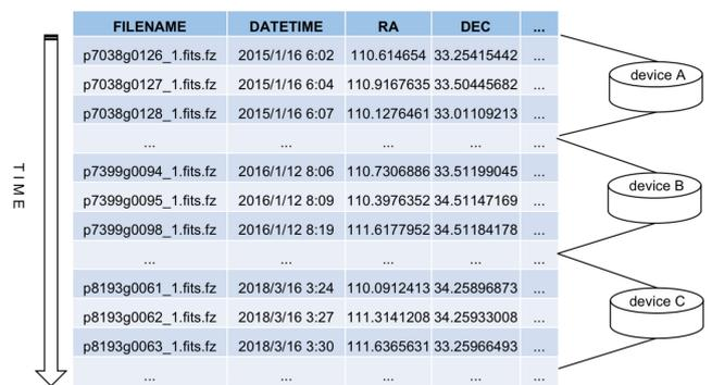
Figure 1: Traditional data placement. The flexible image transport system (FITS) files are organized according to observation time; as such, files labeled with similar observation times are likely to be stored in the same device, whereas the data of specific observation regions may be distributed over multiple devices.
