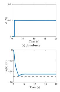
(b) the grasping force  $\lambda_1(t)$  with the disturbance. The response of  $\lambda_1(t)$  without the disturbance is Fig. 2(e).
