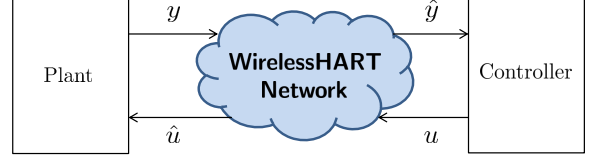
Fig. 3. Block diagram of a NCS over WirelessHART.
