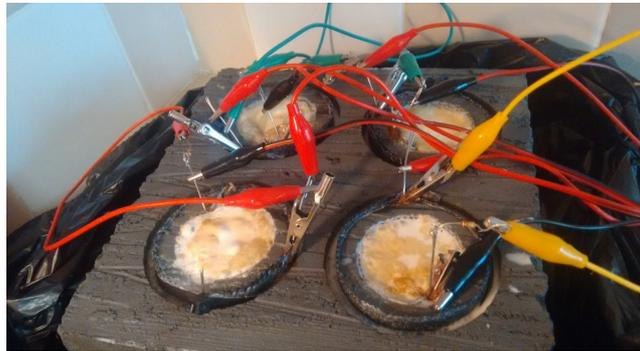
Figure 2: Photo of one block with four aerobic bio-reactors each, in the process of recording electrical potential of the cells.
