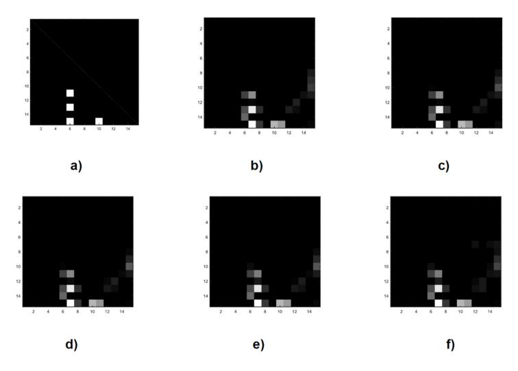
Reconstruction results based on Tikhonov regularization with different thresholds a) the phantom b) SNR threshold is set to 6 c) SNR threshold is set to 7 d) SNR threshold is set to 8 e) SNR threshold is set to 9 f) SNR threshold is set to 10
