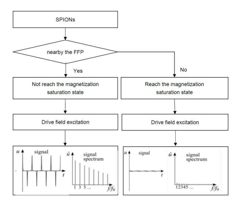
The basic imaging principle of MPI
