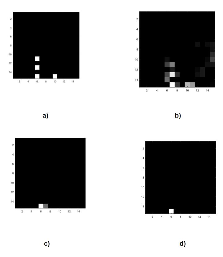
Comparison of the reconstruction results. a) the corresponding phantom b) reconstruction result based on Tikhonov model (-6  $\lambda$  = 5.86 \*10 ) c) reconstruction result based on LASSO regularization ( $\beta$  =0.02) d) reconstruction result based on EN regularization ( $\alpha$ =0.025,  $\beta$ =0.02)
