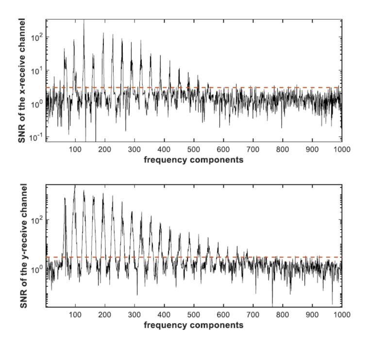
The SNR of the different frequency component for the x- and y-receive channel. The dashed line illustrates the SNR thresholds. (adapted from [6])
