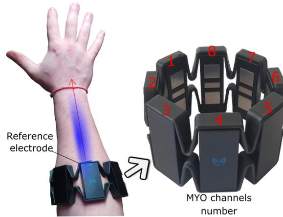
Figure 2: Reference electrode and channels numbers of MYO.
