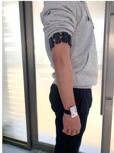
Fig1 Motion Sensor and MYO Arm Ring Wearing Position
