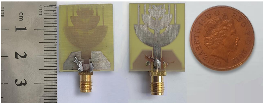
Fig. 4. Fabricated picture of the UWB antenna in the front and back views.
