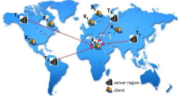
Figure 1: Simplified view of Akamai CDN architecture with four Akamai server regions,  $\{T_1, T_2, T_3, T_4\}$ , and six clients  $\{X_1, X_2, X_3, X_4, X_5, X_6\}$ . Dotted lines show the paths that are monitored for client  $X_6$ .
