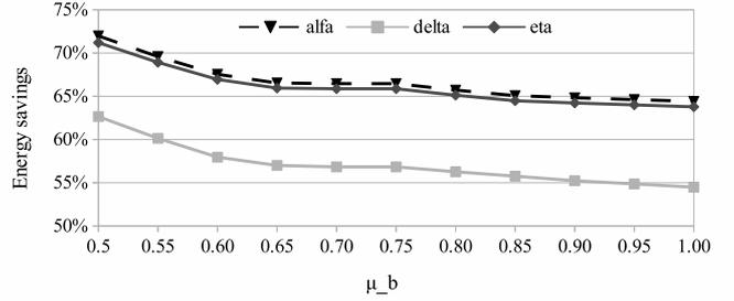
Figure 4: Analysis of the trade-off between energy savings and network congestion, obtained by adjusting the secondary utilization threshold  $\mu_b$  from 0.5 to 1 when solving STPH.
