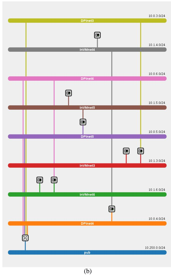
**Fig. 3** Multi-tenant NFV scenario tested on (a) the OpenStack platform and (b) a corresponding virtual network view from the OpenStack platform dashboard. Each tenant slice includes a VM connected to an internal network (InVMnet $i$ ) and a second VM performing DPI and packet forwarding between InVMnet $i$  and DPInet $i$ . The virtual router in the bottom-left corner provides connectivity between each DPInet $i$  and the public network.
